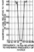
Fig. 22. Sideband filter (HR.22)
