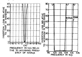
Fig. 10. Carrier filter response Fig. 11. Upper sideband filters (HR.93)
