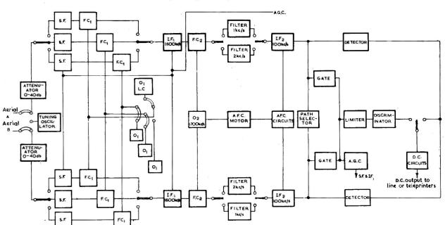
Fig. 2. Simplified diagram of the HR.91
