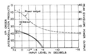
Fig. 8. Fifth order intermodulation products
