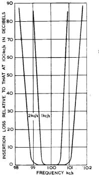
Fig. 4. Filter response (HR.91)
